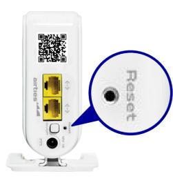
To return the device to factory settings, press down on the reset button (in the small opening on the back shown above) for 5 seconds and release. A metal paperclip (with an extended tip) or strong toothpick are typically good choices for this task. When the reset process is triggered, the LED in the front will “blink rapidly” and the device will reboot to factory settings.
