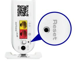
To return the device to factory settings, press down on the reset button (in the small opening on the back shown above) for 5 seconds and release. A metal paperclip (with an extended tip) or strong toothpick are typically good choices for this task. When the reset process is triggered, the LED in the front will "blink rapidly" and the device will reboot to factory settings.
