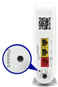
To return the device to factory settings, press down on the reset button (in the small opening on the back shown above) for 5 seconds and release. A metal paperclip (with an extended tip) or strong toothpick are typically good choices for this task. When the reset process is triggered, the LED in the front will “blink rapidly” and the device will reboot to factory settings.
